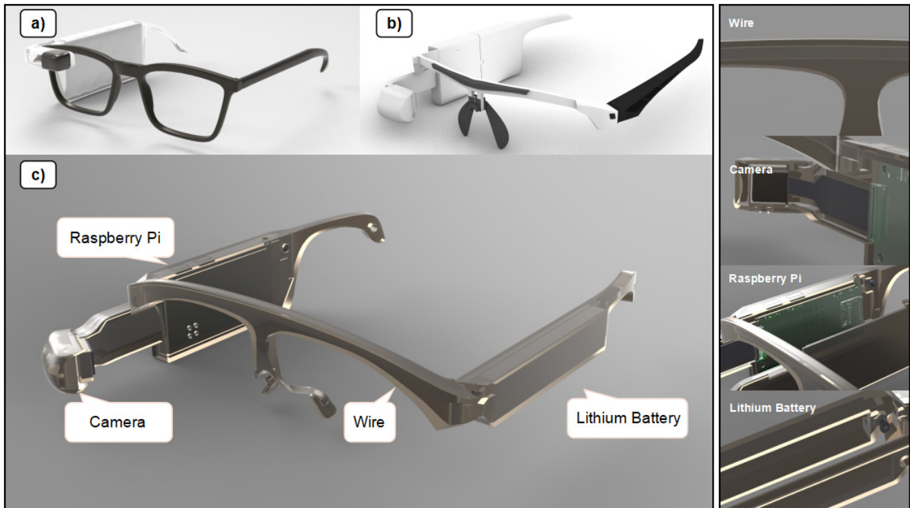
Figure 3: The three eyeglasses prototypes in our iterative design include (a) the first version, in which the frames will block the view; (b) the second version, in which the weight is unbalanced; (c) the final version. The final version contains four main parts: the camera which is used to capture the partial face, the Raspberry Pi which is used to run the ACNN model, and the Lithium Battery which is used to power the system.
