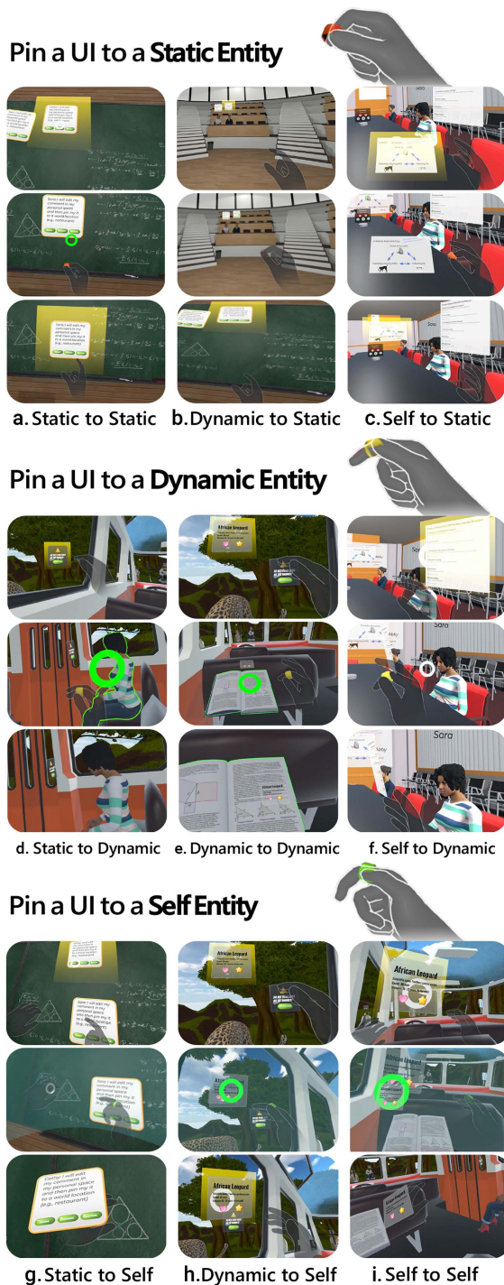
Figure 4: FingerSwitches leverages pinch gestures to pin a UI to a static entity, a dynamic entity, or a self entity in XR. Users first look at and pinch a UI, then look at the target entity, and finally release the pinch to confirm UI transition. Each column (a-i) of screenshots depicts an example application of UI mobility, with detailed descriptions in § 5.2. The green circle indicates the user’s gaze.
