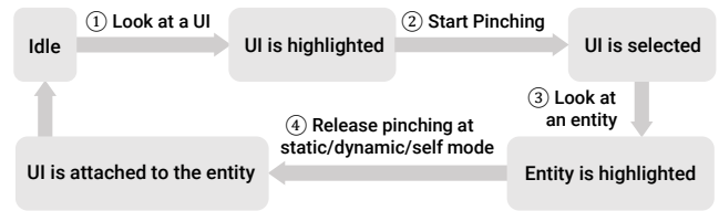
Figure 5: Interaction state transition diagram for FingerSwitches. ① Look at a UI to move. ② Pinch to confirm UI selection. ③ Look at a candidate target entity. ④ Release the pinch. The location on the index finger where the thumb is released determines the mode (“Static, Dynamic or Self”), and the UI will therefore have corresponding positioning and behavior. The interaction is complete and goes back to idle state.
