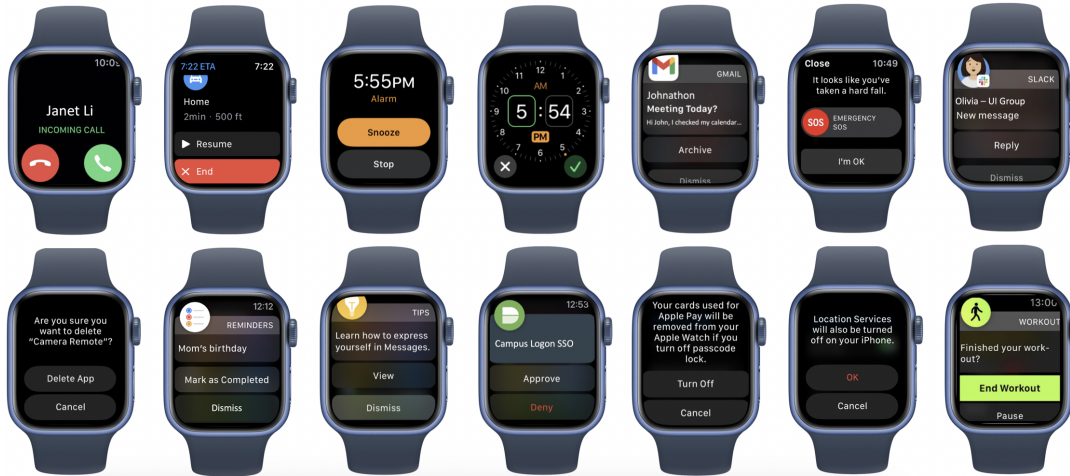
Fig. 1. Examples of confirmation dialogs on smartwatches. First row from left to right: accept/dismiss a phone call, resume/end navigation, snooze/stop an alarm, start/stop an alarm, archive/dismiss an email, start/stop an emergency call, reply/dismiss a message. Second row from left to right: delete/keep an app, confirm/dismiss a reminder, confirm/dismiss a note, approve/deny two-factor authentication, turn on/off a setting, accept/cancel a service change, end/pause a workout timer.
