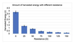
Fig. 3. Investigation of gear ratio's effect on harvested energy (left). Investigation of the effect on harvested energy from the resistance in the motor powerline (right).
