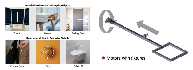
Fig. 1. Translational and rotational motions are the two common types of motion on everyday objects (left). The device designed to simulate these motions on everyday objects and used in the energy investigation tests (right).
