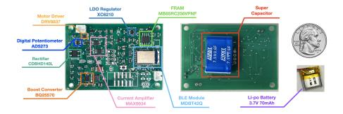
Fig. 5. MiniKers circuit board (front and back).
