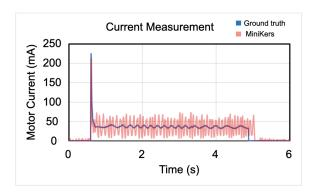
Fig. 10. Comparison of current measurements with MiniKers and Nordic Power Profiler II (ground truth).
