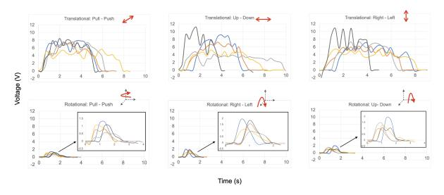
Fig. 2. Signal characteristics of interaction-powered motor mechanisms with two motion types: translational and rotational. Each color denotes data from one participant.
