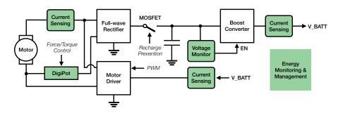
Fig. 6. The power architecture of MiniKers.
