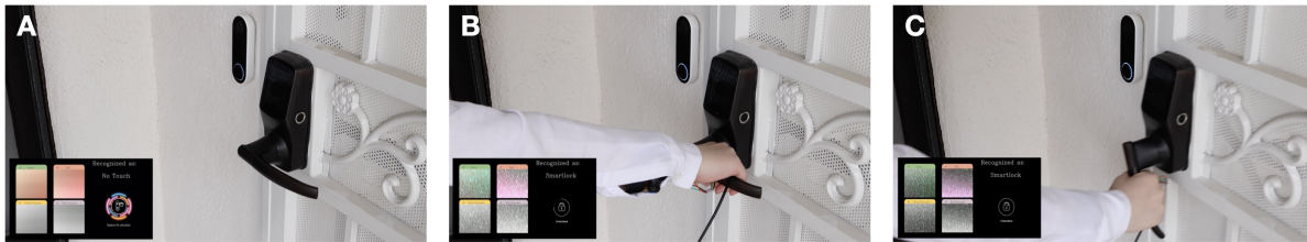
Fig. 17. TextureSight turns a smart ring into keys in authentication applications by detecting its contact with locks with unique textures.
