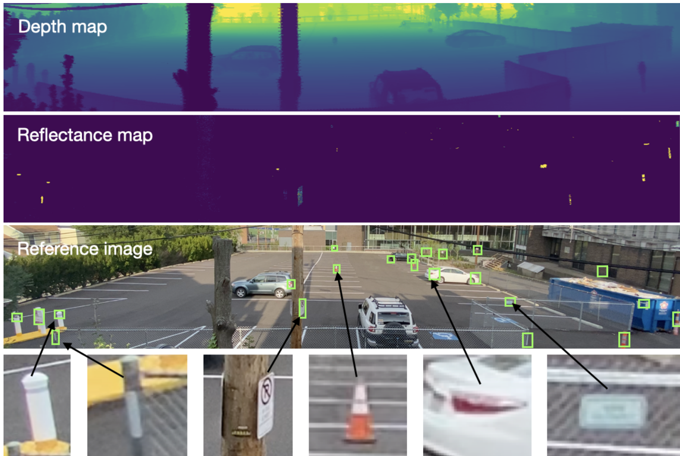
Figure 5: Depth map, reflectance map, and reference image of a parking lot where we conducted the retroreflector search study. Green rectangles denote found retroreflectors.
