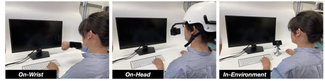
Figure 4: Three sensor locations in the user: On-Wrist (left), On-Head (middle), and In-Environment (right).
