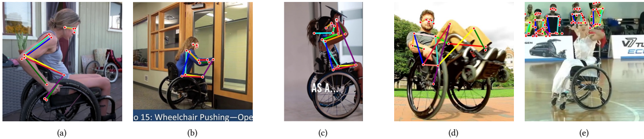
Figure 2: Examples of poor keypoint prediction performance from Detectron2 ImageNet [108]. Figure 2(a) Poor prediction of the legs and torso which are slightly occluded by the wheelchair. Figure 2(b) Both shins are predicted to be on the hand due to the occlusion of the wheelchair. Figure 2(c) Legs are predicted to be on the upper body. Figure 2(d) The right shin is predicted to be on the wheels of the wheelchair. Figure 2(e) The wheelchair dancer is completely undetected by ImageNet.
